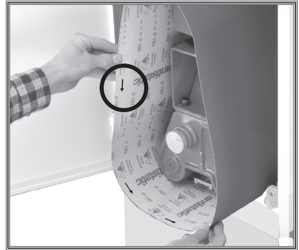
Figure 8. Installing sanding belt over rollers. The arrows on the inside must point in the same direction as belt rotation.
